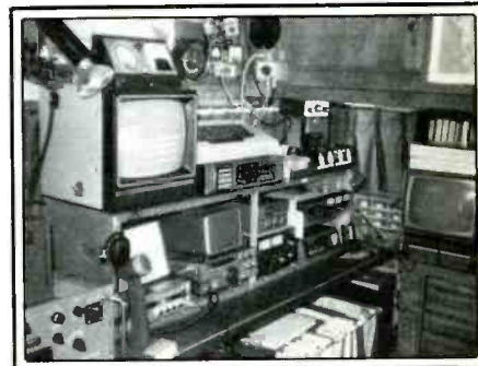
Here is a picture of the equipment installation belonging to Frank Speirling, CA. Frank says it occupies one side of his trailer. The equipment includes a TS430S with antenna tuner, Collins R390A, Info-Tech 600A, UHF scanner 2010, VIC 20 (for logging), Uher tape recorder, 116' dipole antenna for low frequencies, and a Starduster antenna for the higher frequencies.
