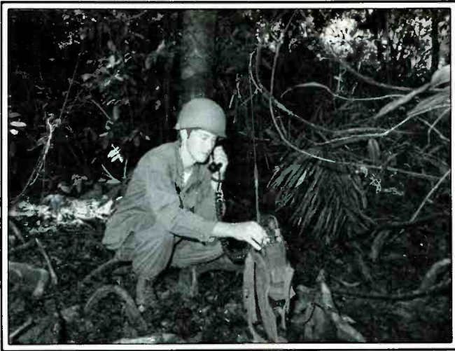
Private First Class Walter Tharp, Analysis Division, U.S. Army Tropic Test Center, Fort Clayton, Canal Zone, operated a portable, manpack radio set in tests to determine frequency propagation of this radio while under heavy jungle canopies and in dense vegetation. (U.S. Army photo.)
